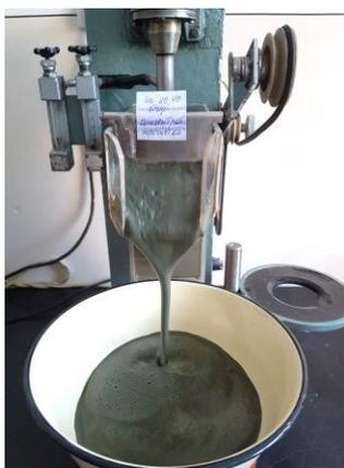
2-rasm. Sulfidli flotatsiya
